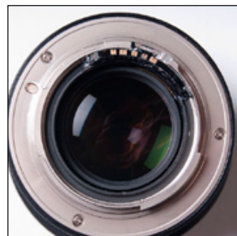
I damaged the very soft metal of the mount when cutting into it to fit the chip shown here. A perfectly clean job should be easy enough.
