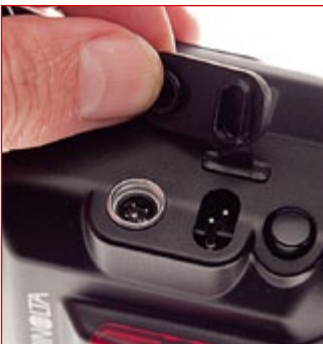
The 58's EX cable and battery pack fittings are identical to the 5600 (below).
