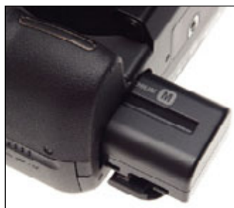
The groove prevents you fitting A100 cells in the 700. The AF-assist for low light returns from the Dynax 7D.
