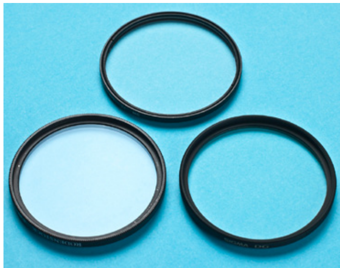
Filter coating effectiveness – B+W MC top, ineffective Rodenstock single-coated lower left, Sigma DG UV lower right with almost 100% effective coating.
