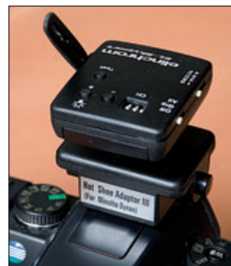
The Elinchrom Skyport RX Transmitter is dedicated to operating the multichannel RX wireless studio flash system. Flash power can be controlled from the camera module.
