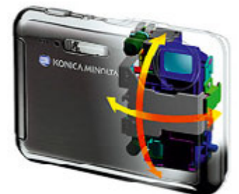
The CCD stays still for Anti-Shake – the lens assembly moves instead.
