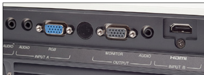
Above: the rear interfaces include S-Video (out of shot, left) D-Sub 15 pin computer in and out, and HDMI (right) which carries audio as well as picture. Below: the top buttons are very easy to use. Projected menu instructions help too.
