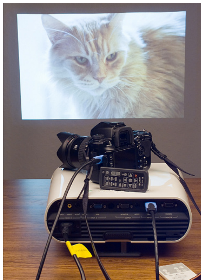
The Alpha 900 is shown on top of the projector to make the connection (mini-HDMI to HDMI) cable and remote controller visible. Normally you sit the camera facing you, so the remote can control image changes and zooming in (above right).
