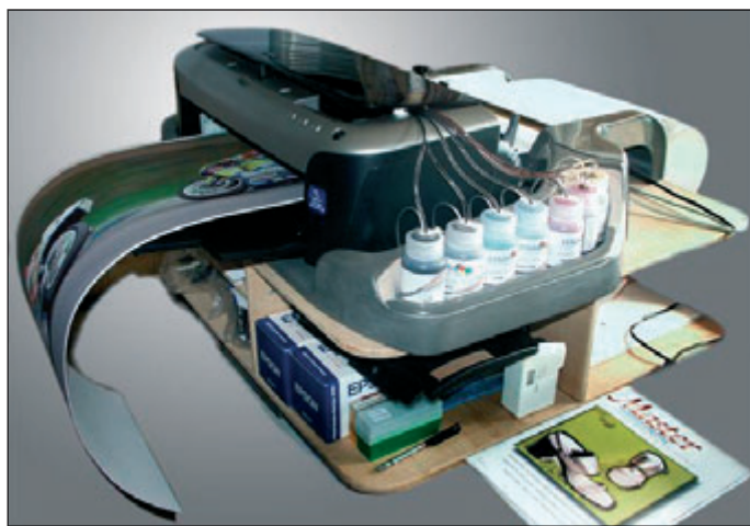
This is one of Cliff Carter's set-ups for supporting long cut sheets of panoramic paper, on an Epson 2100 A3 printer equipped with a Lyson continuous ink supply. The A4 magazine shows the scale of the assembly. Some printers accept roll feed paper which can be used for 3.5 inch wide panoramic output.
