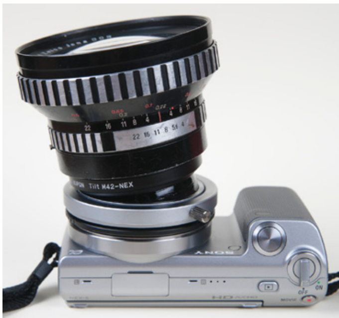
The very old and scruffy 20mm f 4 Flektogon mounted on the Kipon M42 thread tilt adaptor for NEX. This lens has a stop-down lever. You can not use similar lenses without a stop-down method unless you tape the aperture pin down.
