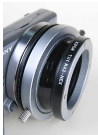
The Kipon tilt adaptor is a ball and socket based design with a clamping screw ring. The amount of tilt is not marked in degrees, but is very similar to dedicated tilt lenses. Kipon is also introducing tilt-shift adaptors for medium format lenses used on SLR bodies. C/Y, Leica R, and Nikon mount adaptors are also available.
