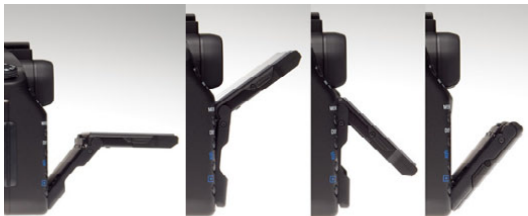
Four positions of the Alpha 300/350 rear screen – intermediate angles are possible. It can not turn round to face the front, or be angled out to the side for portrait format shots.
